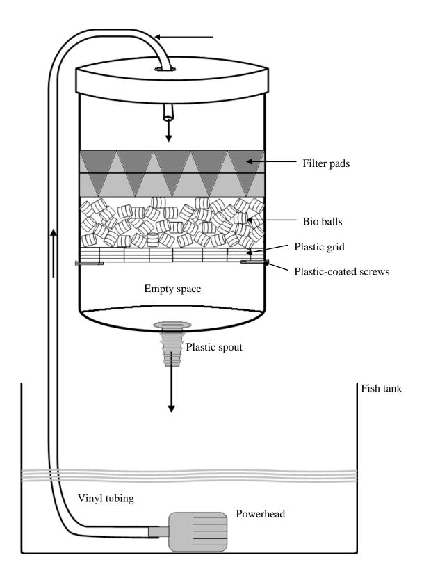
Figure 2. Bucket biofilter.
